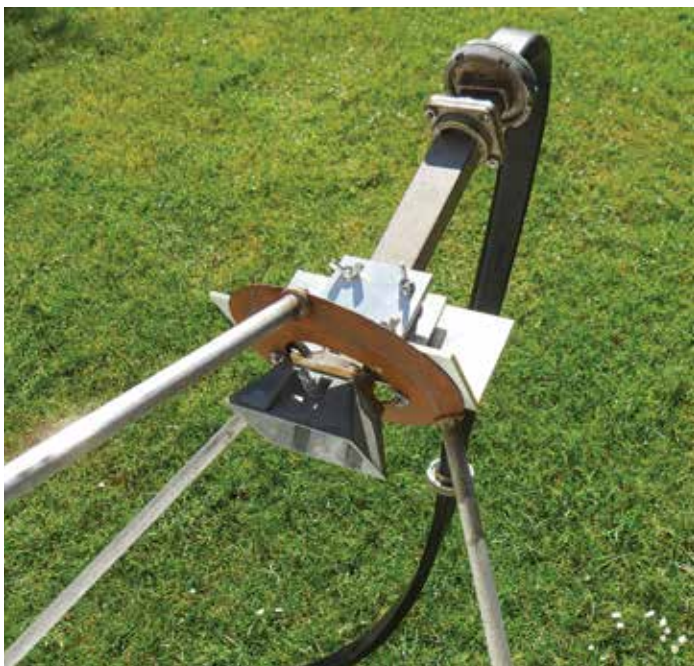
PHOTO 4: An example of a horn antenna dish feed used on the 3cm band to receive a signal using the 1200mm dish.
