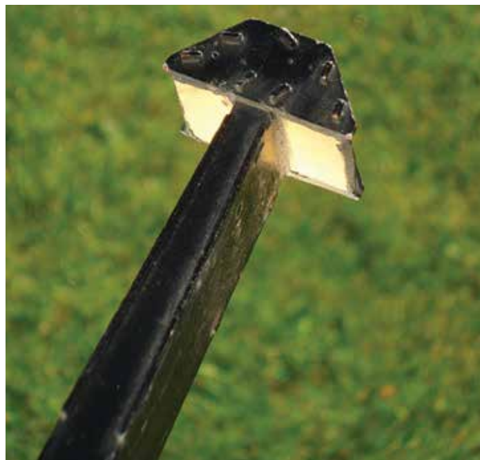
PHOTO 5: An example of a waveguide fed horn dish feed used on the 3cm band to receive a signal using the 750mm dish.
