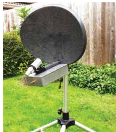
PHOTO 6: An example of an offset fed dish using a conical horn dish feed used for terrestrial 3cm band contacts.
