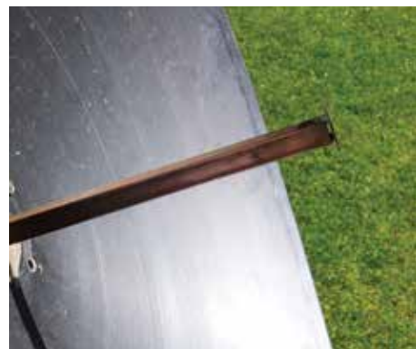
PHOTO 7: An example of a waveguide 'penny' dish feed used on 47GHz.
