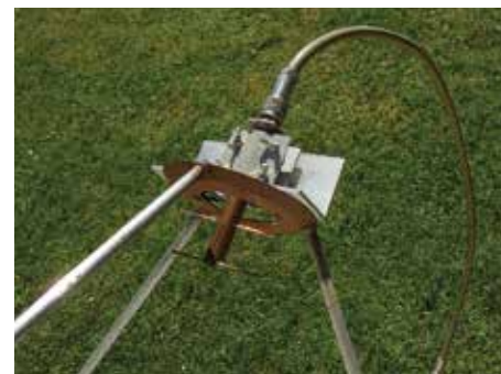
PHOTO 3: An example of a dish feed used on the 13cm band to transmit a signal using the 1200mm dish. The two element dish feed beams a signal toward the dish.
