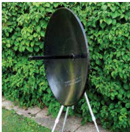
PHOTO 2: A 750mm diameter dish used to receive the QO-100 satellite on the 3cm band. This dish gives around 36dB of gain at this wavelength.
