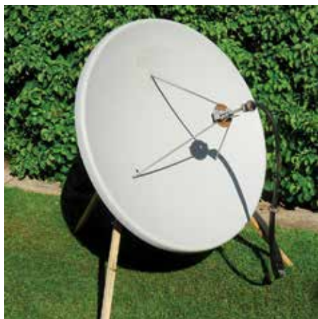
PHOTO 1: A 1.2m diameter metal-covered fibreglass dish set up to receive the QO-100 satellite on the 3cm band. This dish gives around 40dB of gain at this wavelength.
