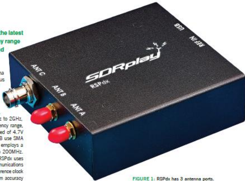
FIGURE 1: RSPdx has 3 antenna ports.
